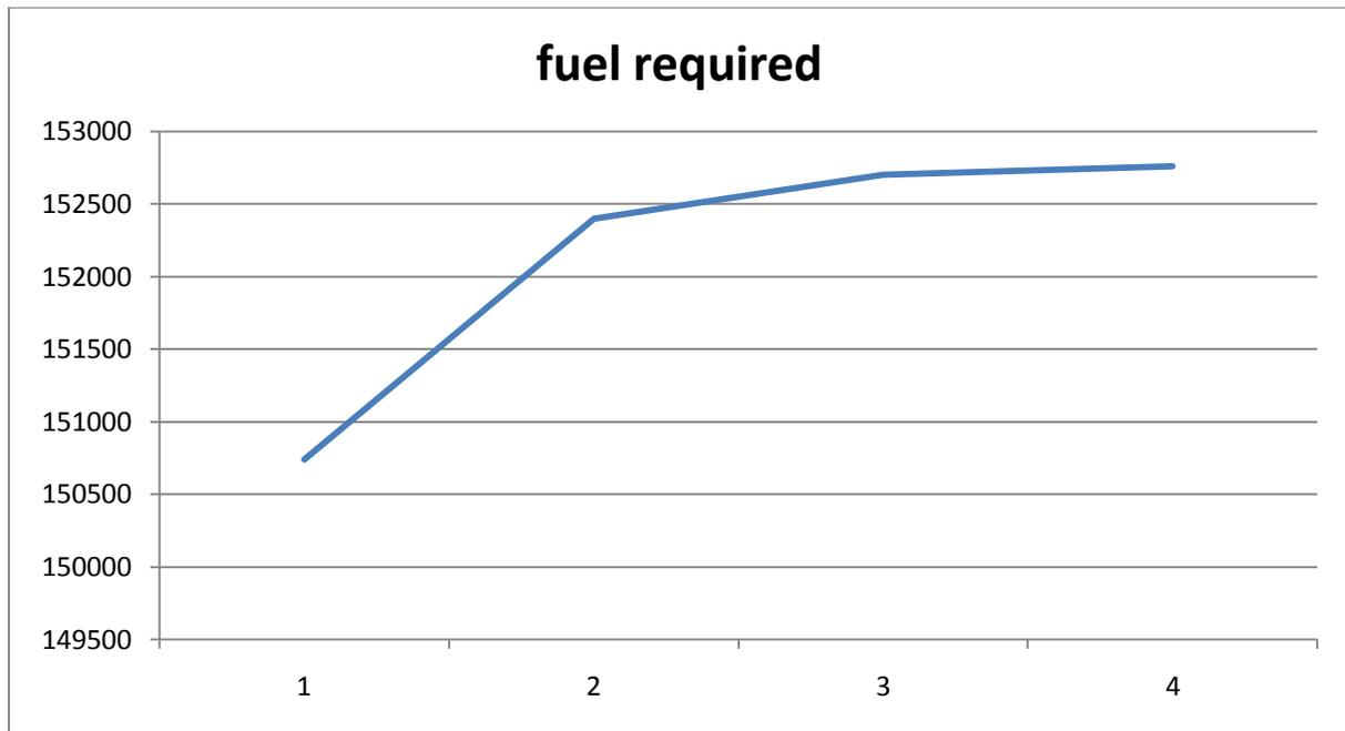
The graph will continue to level out indefinitely. As more fuel is added, more fuel must be added to compensate for the increase in weight. This addition of fuel as decreased through each cycle because of the constant mass of the rocket with no fuel.
