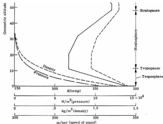
From the altitude ( $h$ ) to density ( $\rho$ ) graph on the left, a model was developed to determine the average density for the troposphere and the stratosphere.
